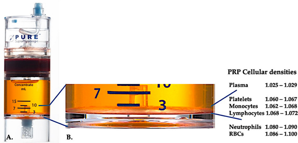
Figure 1. Cellular density separation of whole blood following a two-spin centrifugation procedure using the PurePRP-SP ® device (EmCyte Corporation, Fort Myers, FL, USA). After the first centrifugation procedure, the whole blood components are separated in two basic layers, the platelet (poor) plasma suspension and the RBC layer. In A, the second centrifugation step has been completed. The factual needed PRP volume can be extracted for patient application. The magnification in B shows at the bottom of the device the organized multicomponent buffy coat layer (indicated by the blue lines), containing high concentrations of platelets, monocytes, lymphocytes, based on density gradients. In this example, a minimal percentage of neutrophils (<0.3%) and RBCs (<0.1%) will be extracted, following a neutrophil poor C-PRP preparation protocol.
